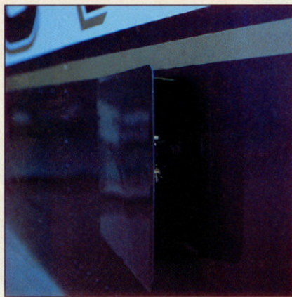
The 98-pound air conditioning system runs off its own 135-amp alternator and uses a large fuselage-mounted intake door.
