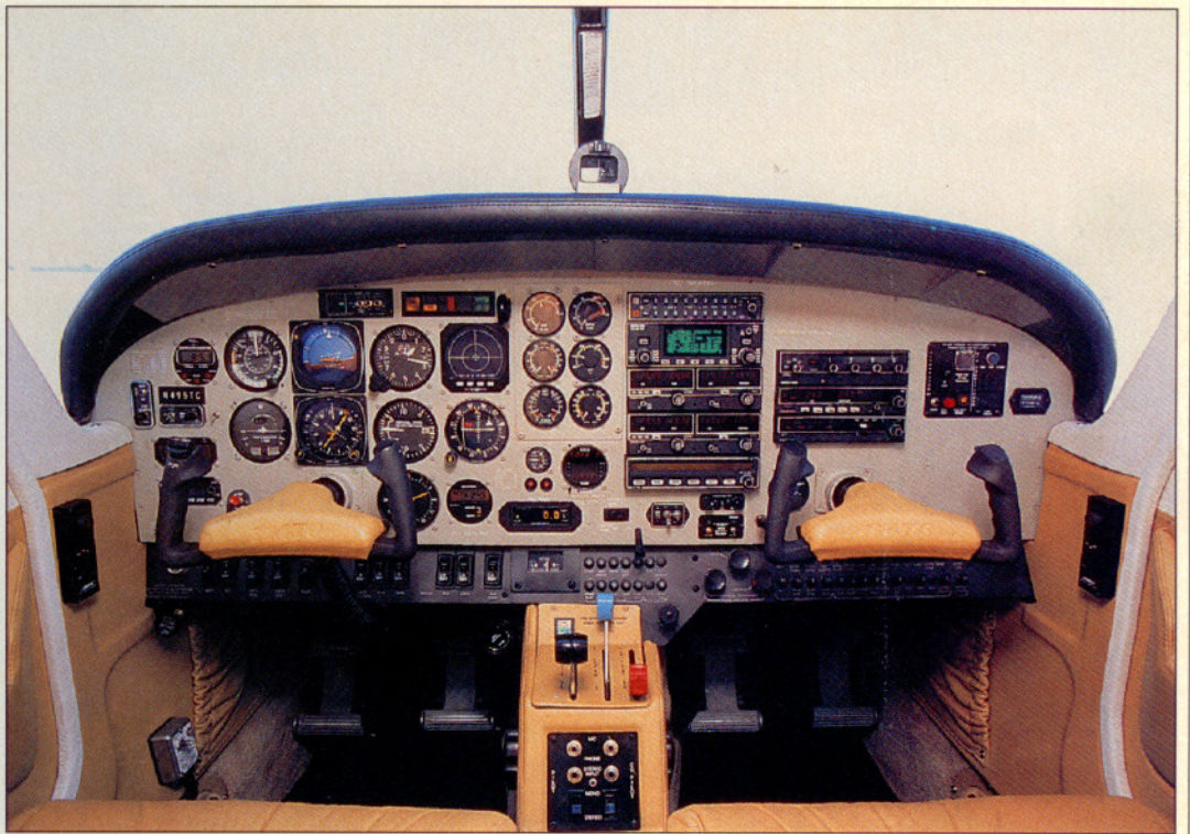
A large, well-equipped panel including GPS, autopilot, optional oxygen, and lightning detection equipment rounds out a cavernous and comfortable interior (above). Below, the turbocharged Lycoming TIO-540 puts out 270 hp at a quiet 2,575 rpm. Engine temperature control is aided by a pair of electrically actuated cowl flaps.
